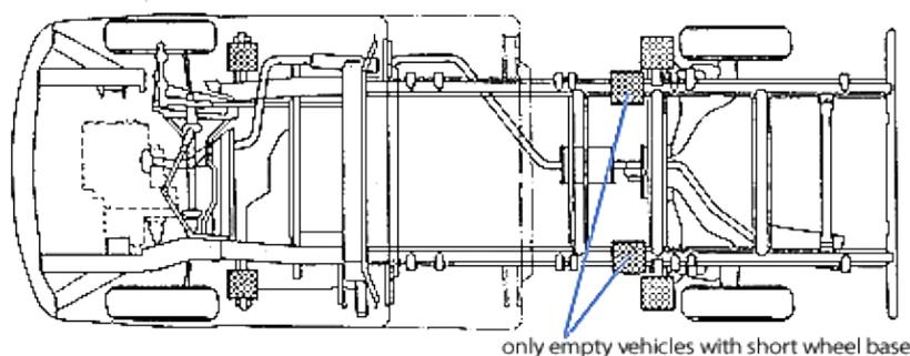
a) 4 location points are shown in front of the rear axle. The note "Only for empty vehicles with short wheel base" indicated below, only applies to the two location points at the side rails.
