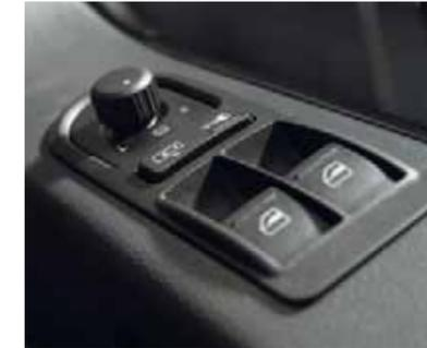
**Control unit for electric door mirrors, windows and central locking.**
