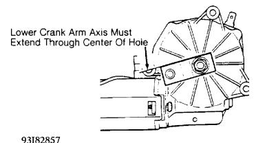
Fig. 2: Aligning Rear Motor Crank Arm (EuroVan) Courtesy of Volkswagen United States, Inc.
