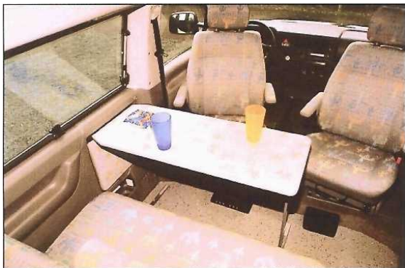
The full-sized table is rather narrow but it is extremely solid with its single leg located in the sliding seat's floor channel.
