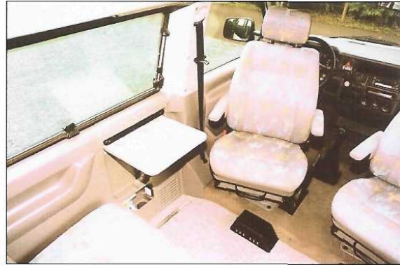
A small coffee table simply hinges up from the side wall for use. At floor level the black vent is the blown-air heating outlet.
