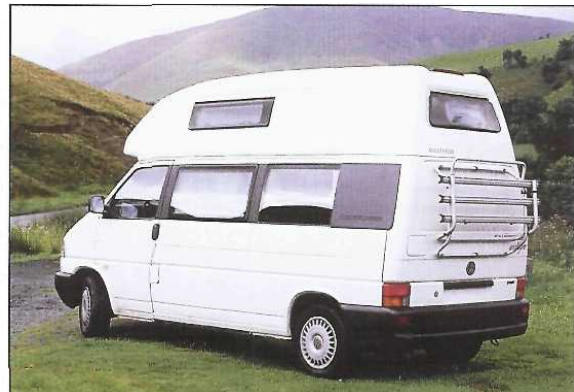
The 'upstairs' bed is ready in an instant and has unusually generous headroom. Lighting, opening windows and stereo speakers are all fitted in the roof.
