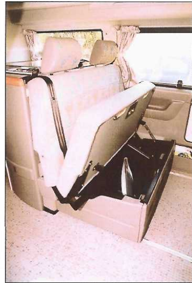
Stowage space is available under the rear seat. The squab tips up for access and is supported by a strut.
